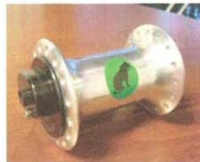
Pantour Rocklite front suspension disc hub 1 inch travel, 100 mm axle Rohloff 4 bolt rotor
